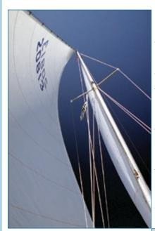
mast's height. A single spreader will be in the middle of the mast. Special rigging between the mast and spreaders takes pressure off the mast itself.
